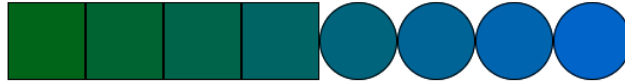
Figure 2.1: Enter and exit example for D3, using the code shown in Listing 2.3. Rectangles are already existing DOM-elements from the last iteration while circles are freshly created DOM-elements during the current iteration.
