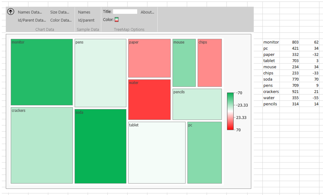
Figure 5.4: A treemap visualisation using the Treemap Excel app. The rectangle labels are mapped to the values in the first column, the size is mapped to the values second column and the colour is mapped to the values in the third column.
