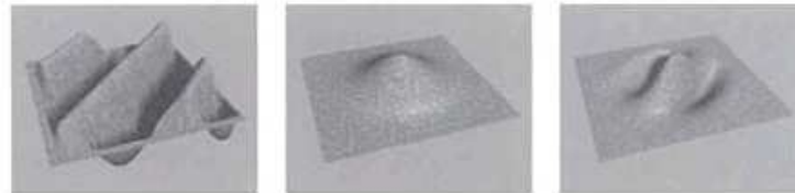
Figure 4.2: 1st is the cosine field, 2nd is the Gaussian field and 3rd is the Gabor field composed from the 1st and 2nd field by multiplying Ware [2004].
