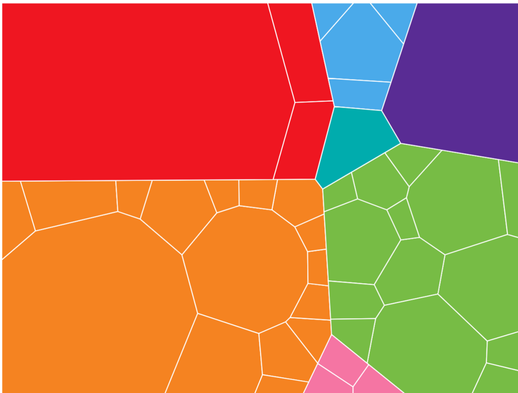
Figure 2.3: A Treemap using a Voronoi Diagram in each level of the hierarchy. This visualization is called a Voronoi Treemap. Different colors are used to make the different cells easily distinguishable.
