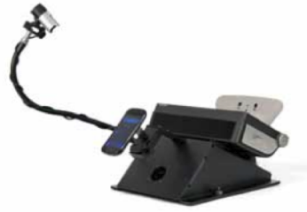
Figure 4.3: Tobii Mobile Device Stand with Tobii Scene Camera and Tobii Eye Tracker [29]
