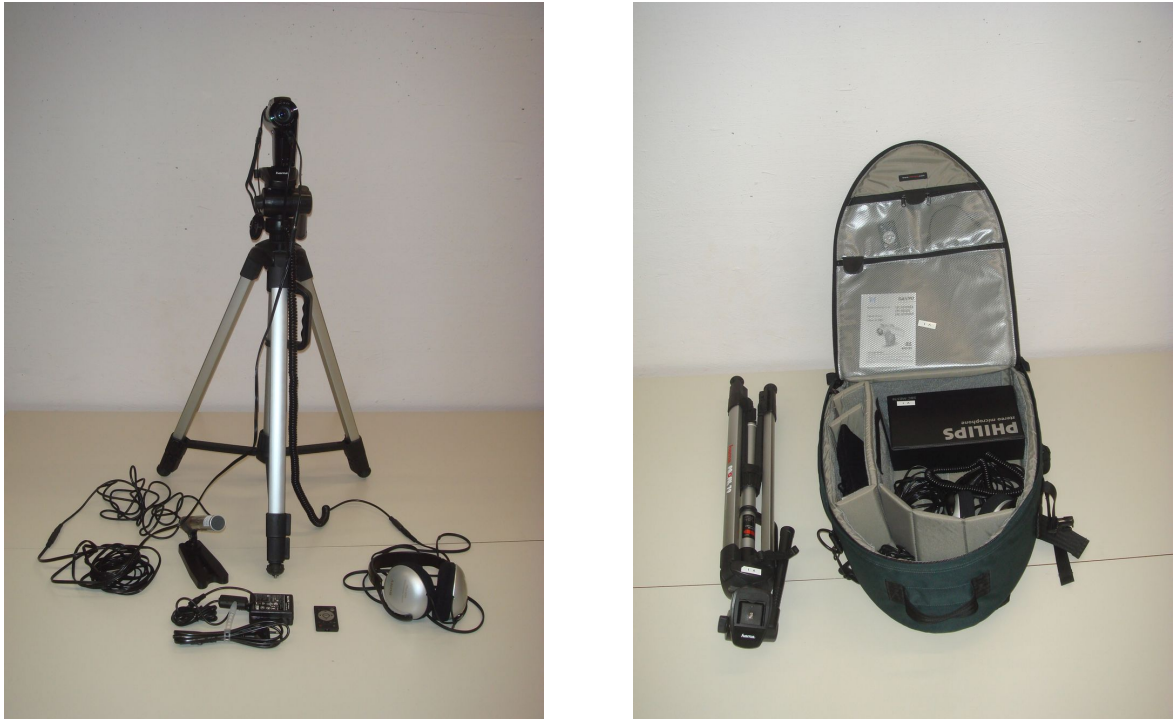
Figure 9.13: The portable usability kit used at Graz University of Technology. On the left the kit has been set up ready for use. The righthand photos illustrate packing the kit.
