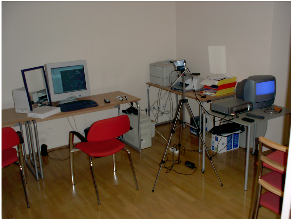
Figure 9.3: Simple usability test setup in 2002 with a single video camera. A mirror is used to capture the user's facial expressions. Video is recorded onto a VHS cassette.
