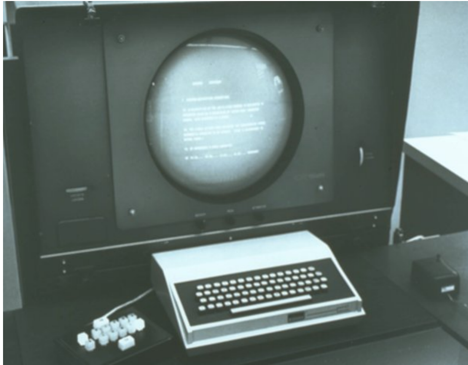
Figure 13.4: An NLS workstation with a CRT display, keyboard, push buttons, and mouse. [ Image used with kind permission of Stanford University, Special Collections. ]
